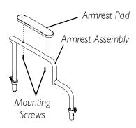
FIGURE 7.3 Replacing Armrest Pad
